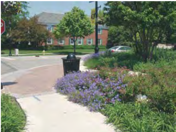
Varying the location of the sidewalk at corners can create additional areas for landscape. Changing the paving materials at intersections and in crosswalks helps motorists and pedestrians identify when they are approaching pedestrian first areas.
